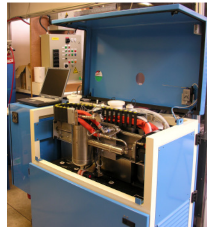
5 kW HOD Hydrogen generator
